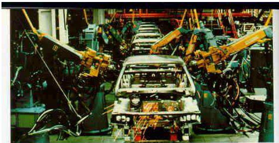
Industrial robots spot weld automobile bodies on an assembly line.
